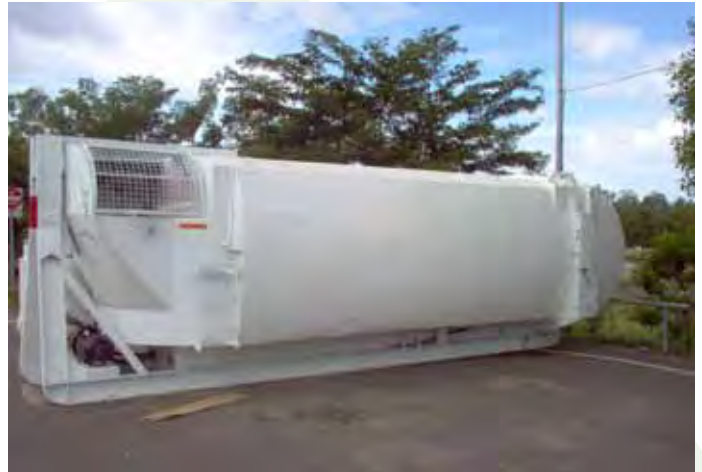
■ One of the three former collection trucks which is now being used as a stationary compactor for cardboard.
