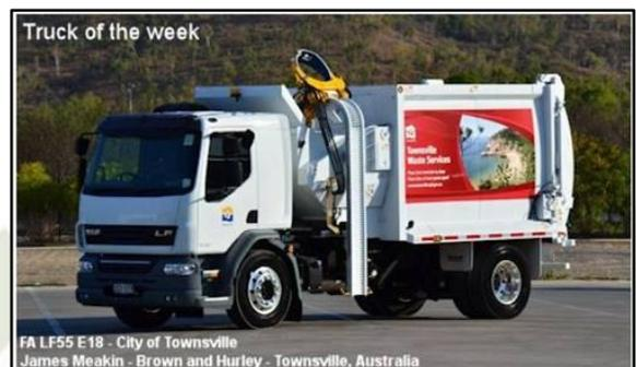
The design of the lifting arm allows the truck to access narrow streets and service lanes more easily to conduct services, lessening the risk of strike to surrounding buildings, fences and other obstructions.
